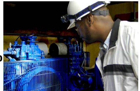
Provides hands-free lighting for the worker when there is no place to put a light
