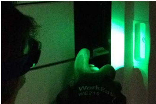
Green LED feature allows night crews to work outside and does not attract flying insects or spook wildlife
